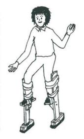
Main uprights: 2"x1" wood for children. 3"x1" for adults. Reaches up to knee. Foot platform: 3" ply, approx. foot size, screwed and glued to support. Platform support: 2"x2" or 2"x3" BOLTED to upright. From ground to platform about 18" for starters, up to 30" for experts. Foot made from 4 pieces of 2"x1", screwed together and bolted to upright. Tack a piece of rubber mat or tyre to the bottom for grip.
