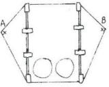
3. Reinforce the "bridle-points" (A + B) with tape and make a small hole in each.
